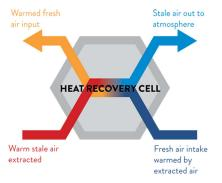
For residential buildings, utilising a Mechanical Ventilation with Heat Recovery (MVHR) system provides the greatest energy benefit by reducing winter heat loads. However, there are alternative ventilation systems which do provide some demand control over air infiltration. These should only be considered where MVHR systems are shown by the applicant to be beyond the viability of the project.
